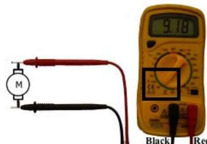
Figure 4.3: Connecting the DMM to the Motor
