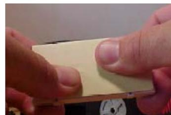
Figure 3.2: Seating a protoboard's contacts
