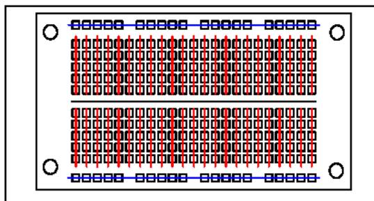
Figure 3.3: Arrangement of nodes and buses on a protoboard
