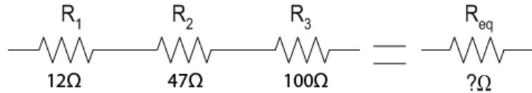
Figure 3.11: Resistors in Series
