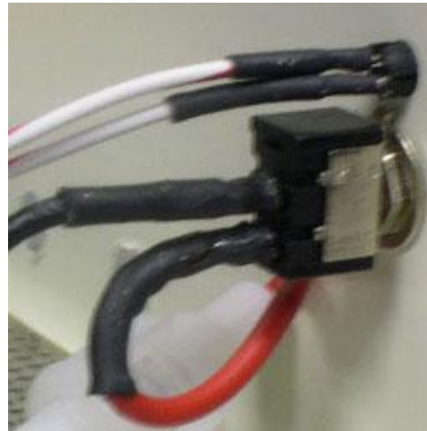
Figure 8: Safely made connections for high voltage
