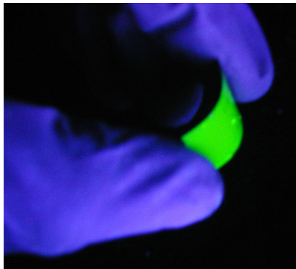
Figure 1: A 450 nm thick film of Zn 2 GeO 4 :Mn deposited on a flexible polyimide substrate shows bright green PL after hydrothermal annealing.
