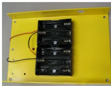
Figure 2.19: Full view of Battery Holder
