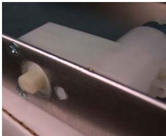
Figure 2.23: Motor being mounted on TekBot frame
