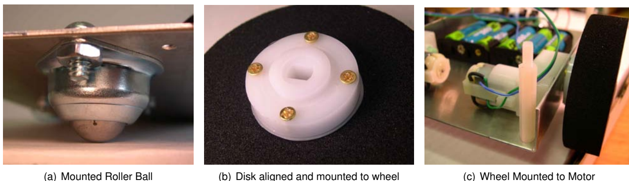
Figure 2.25: Assembly of Roller Ball and Wheels
