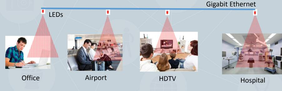
Coverage area: 2D-array of optical transmission cones
